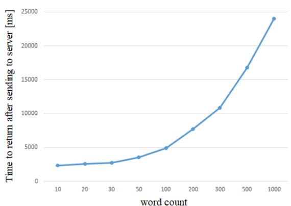
Fig. 13. Measurement results for time by data size (returning to the client through the server)
