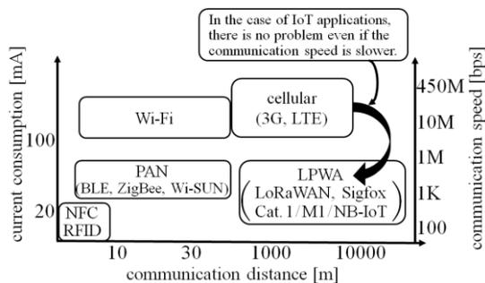
Fig. 1. Relationship between communication speed and power consumption
