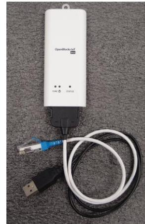
Picture 4. Sensor data receiver (OpenBlocks IoT BX0)
