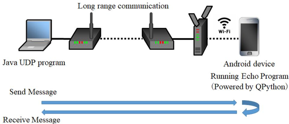
Fig. 11. Transmission/reception test using echo program
