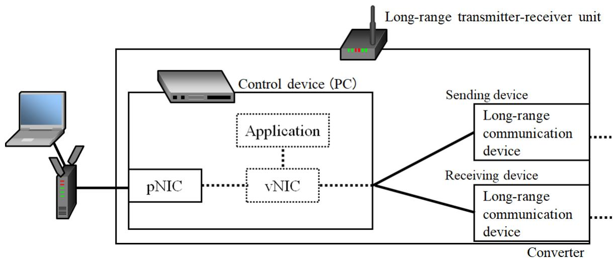
Fig 3. Components required for long range communication
