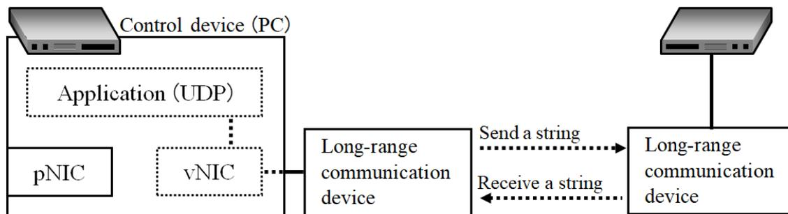
**Fig. 6. Measuring the time needed to receive the sent string again (echo Server)**
