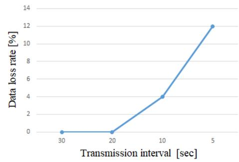
Fig. 14. Data loss due to transmission interval
