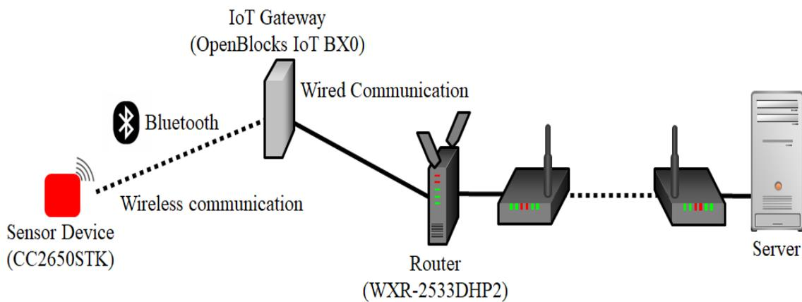
Fig. 7. Transferring sensor device data to remote servers
