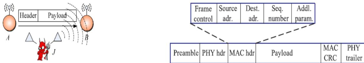
Fig. 1 Recognition of a selective jamming attack and a general frame format in a wireless network
