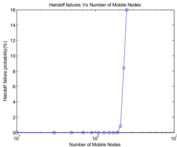
Figure 6. HO failures probability vs. number of MNs
