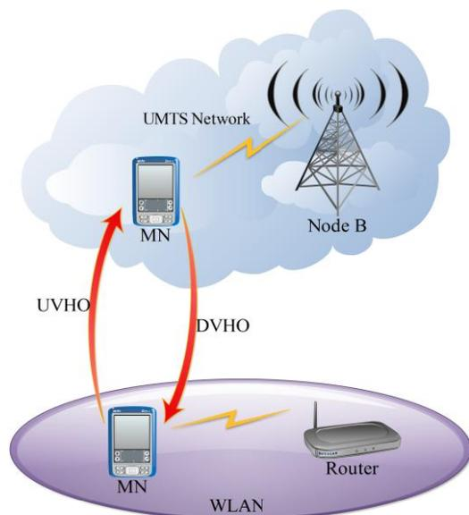
Fig. 2 Upward and Downward VHO
