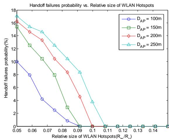
Figure 5 HO failures probability vs. Relative size of WLAN Hotspots ( $R_w/R_u$ )
