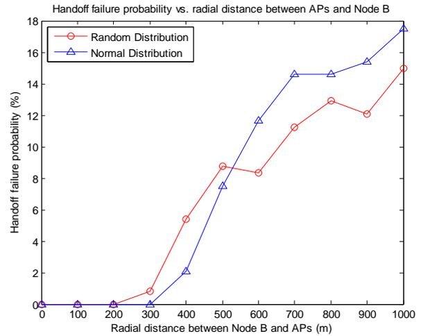
Figure 4 HO failures probability vs. radial distance between APs and Node B ( $D_{AP}$ )
