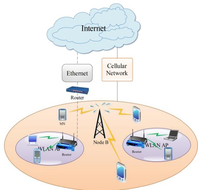
Fig. 1 Two-tier Heterogeneous Network
