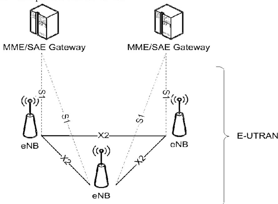
Fig.1 LTE architecture with E-UTRAN
