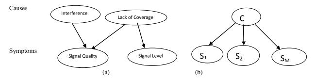
Fig. 2.0 Example of Bayesian Network for Diagnosis in Cellular Networks and Simple Baye's Model
