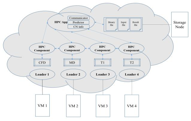
Figure 4. The Proposed adaptive high-performance Execution framework.
